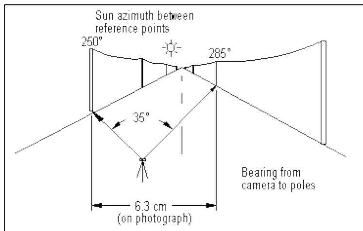
Figure 7. Horizontal Scaling.
